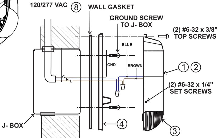
Product is supplied assembled. To separate Housing and Base, remove two #6-32 screws at top of housing and back out two #6-32 set screws on each side.
