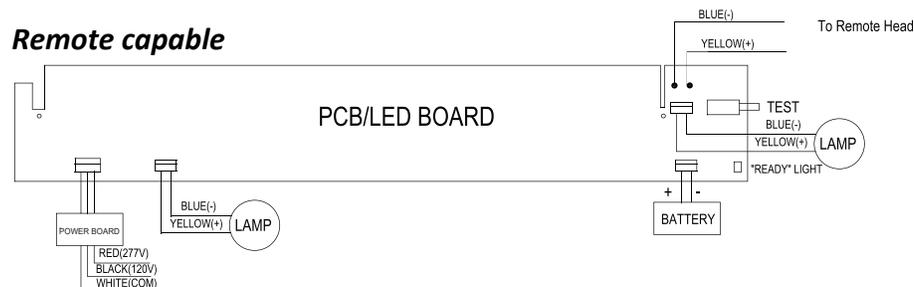
**CAUTION:** DO NOT connect YELLOW and BLUE remote leads together. Please also ensure remote head positive (+) lead is connected to COMBO unit's yellow lead (+) and remote head negative (-) lead is connected to COMBO unit's blue lead (-).
